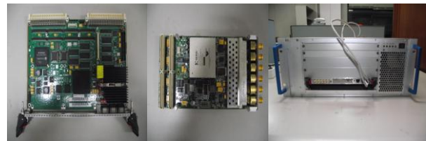
Fig. 4 The Physical Hardware used in VME Configurations
